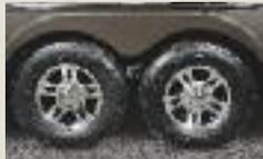
Premium E-rated tires are standard on all models with 8-lug, easy lube axles and aluminum alloy wheels.
