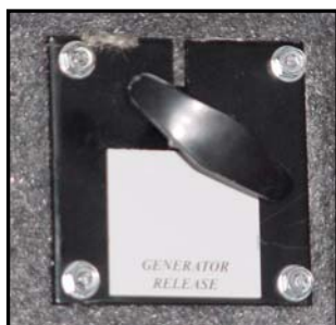
Figure 7-18. Generator “Pull” Cable Slide-Lock Release
