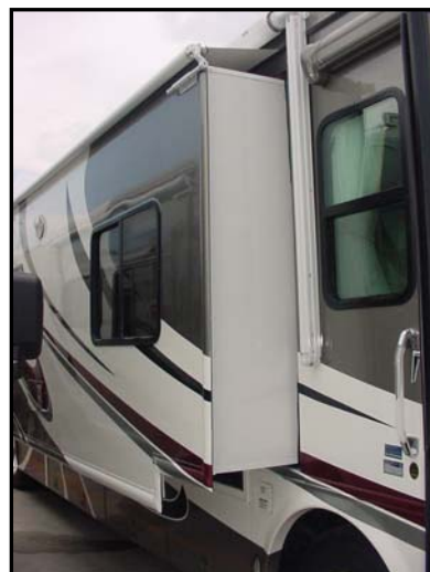
Figure 8-2. Typical Slide-Out Fully Extended
