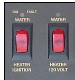
Figure 4-17. Water Heater Switches
