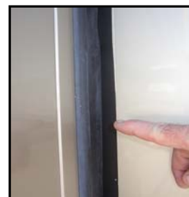
Figure 14-6. Inspecting Slide Out Gasket
