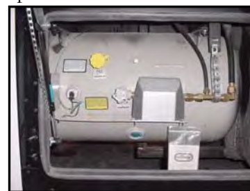
Figure 2-4. Liquid Propane Tank
