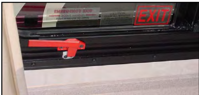
Figure 12-2. Bedroom Emergency Exit Window
