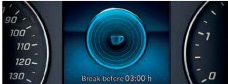
**ATTENTION ASSIST®** helps prevent drowsy driving by monitoring your driving patterns and providing an early warning in case fatigue is detected.
