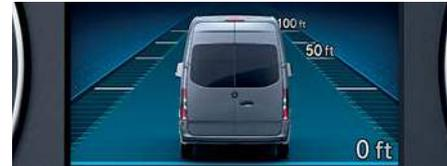
**ACTIVE DISTANCE ASSIST DISTRONIC®** is an intelligent cruise control system that senses traffic conditions and actively controls your speed to keep you at a safe distance.
