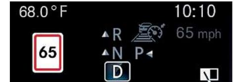
**TRAFFIC SIGN ASSIST** uses a camera to give drivers additional help with identifying speed restriction signs, No Passing Zones, and No Entry signs.
