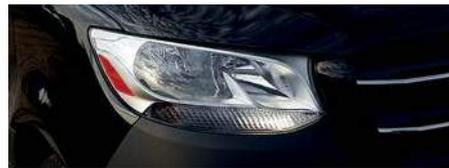
**HIGHBEAM ASSIST™** adjusts the high and lowbeam headlamps automatically, allowing for continuous adaptation to the prevailing traffic situation. The system helps ensure better and earlier recognition of the course of the road.
