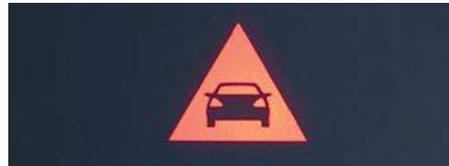
**ACTIVE BRAKE ASSIST** is an advanced system that senses the likelihood of a collision with a vehicle ahead and sends both a visual and audible warning followed by initiating autonomous braking.
