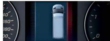
**ACTIVE LANE KEEPING ASSIST** can provide you with visual and audible warnings if your van leaves its lane unintentionally. A camera in the windshield monitors the road ahead and helps detect when you may have veered away from lane markings. There is an active element that will center you back in the lane if you cross the outside solid lines. This is accomplished with vector braking. This feature can help prevent vehicles from ending up in ditches or down a mountainside.
