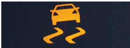
**LOAD-ADAPTIVE ELECTRONIC STABILITY PROGRAM (ESP®)** is a dynamic handling system that actively intervenes to help keep the van firmly under control and safe by automatically braking individual wheels and reducing engine power to help stabilize the vehicle if wheelspin, understeer, or oversteer is detected.
