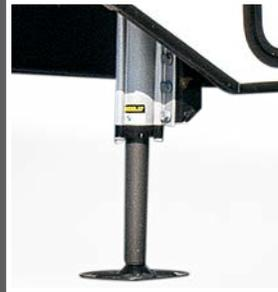
**STANDARD 6-POINT HYDRAULIC AUTO-LEVELING SYSTEM** does all the work
