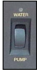
Figure 11-5. Water Pump Switch
