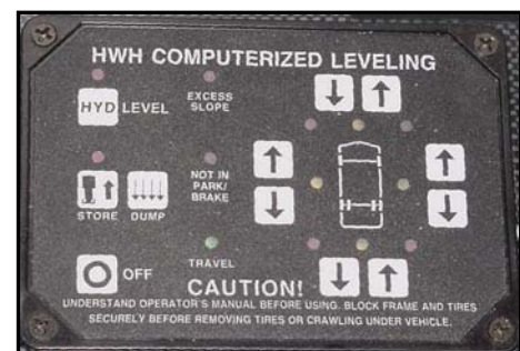
Figure 9-5. HWH Computerized Leveling System
